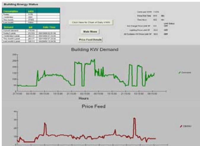
Electricity Consumption (that is on the top in green) vs Electricity Cost (that is on the bottom in red) Consumption vs Cost.
